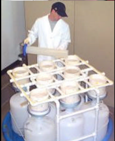
Soil column experiment for study of contaminant mobility
